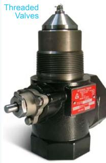
Cavagna threaded valves are compact and can be operated either manually or remotely via cable or pneumatic control. The valves contain spring loaded PTFE packing providing excellent leakage protection and the standard disc material is Nitrile.
