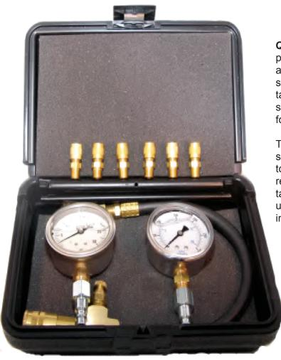
QTG Kits include a 30 psi and a 300 psi gauge, six pressure tap valves, a high pressure test block and a hose assembly. The hose assembly has an inlet swivel connection for attachment to the pressure tap valve and the outlet connection is a high pressure (300 psi) industrial quick disconnect coupling for attachment to either the 30 psi or 300 psi gauge.
